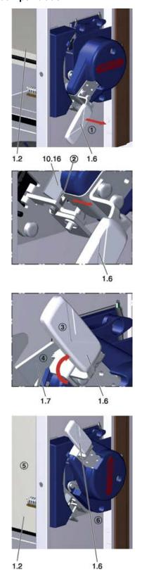
Fig. 172: Close the damper blade
