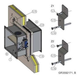
Fig. 27: Fastening the installation kit to the metal studs
