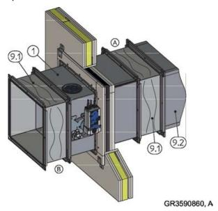
Fig. 162: Fire damper with flexible connectors
