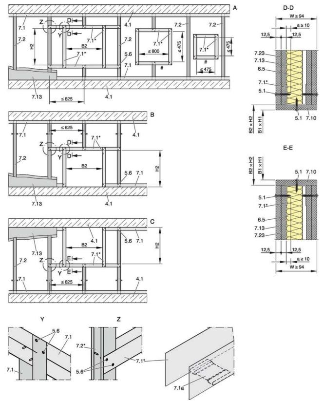
Fig. 65: Lightweight partition wall with metal support structure and cladding on both sides, explanation see Fig. 66
