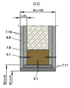
Fig. 91: Lightweight partition wall, half-timbered construction with cladding on both sides
