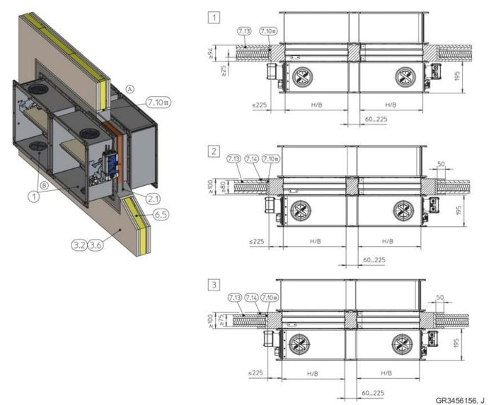
Fig. 71: Mortar-based installation into a lightweight partition wall, flange to flange, illustration shows side by side installation (applies also to installation of dampers on top of each other)
