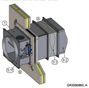
Fig. 163: Fire damper with circular spigots
