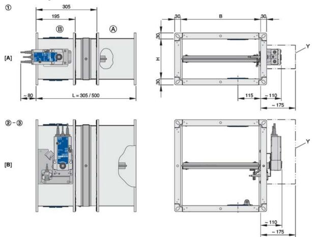
Fig. 5: FKA2-EU with Belimo spring return actuator
