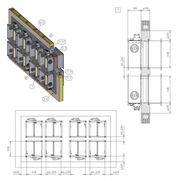
Fig. 101: Mortar-based installation – multiple installation into one installation opening in a timber stud wall
