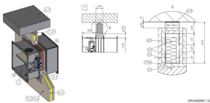
Fig. 74: Mortar-based installation into a lightweight partition wall, below a flexible ceiling joint
