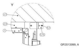
Fig. 26: Installation kit – clear space, for installation near the floor or ceiling
