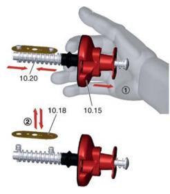
Fig. 180: Replacing the fusible link
