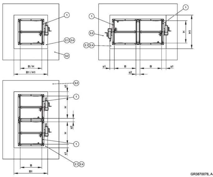
Fig. 64: Lightweight partition walls with metal support structure – arrangement/distances
