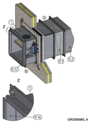
Fig. 165: Fire damper with connecting subframe
