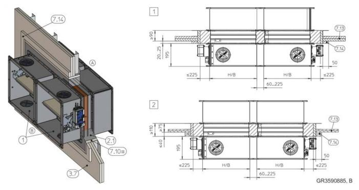
Fig. 123: Mortar-based installation into a shaft wall, flange to flange, illustration shows side by side installation (applies also to installation of dampers on top of each other)
