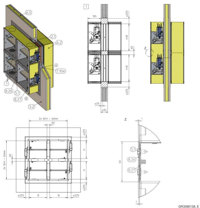
Fig. 77: Mortar-based installation – 4 dampers with a common duct
