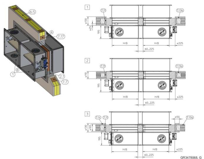
Fig. 93: Mortar-based installation into a lightweight partition wall with timber support structure, flange to flange, illustration shows side by side installation (applies also to installation of dampers on top of each other)
