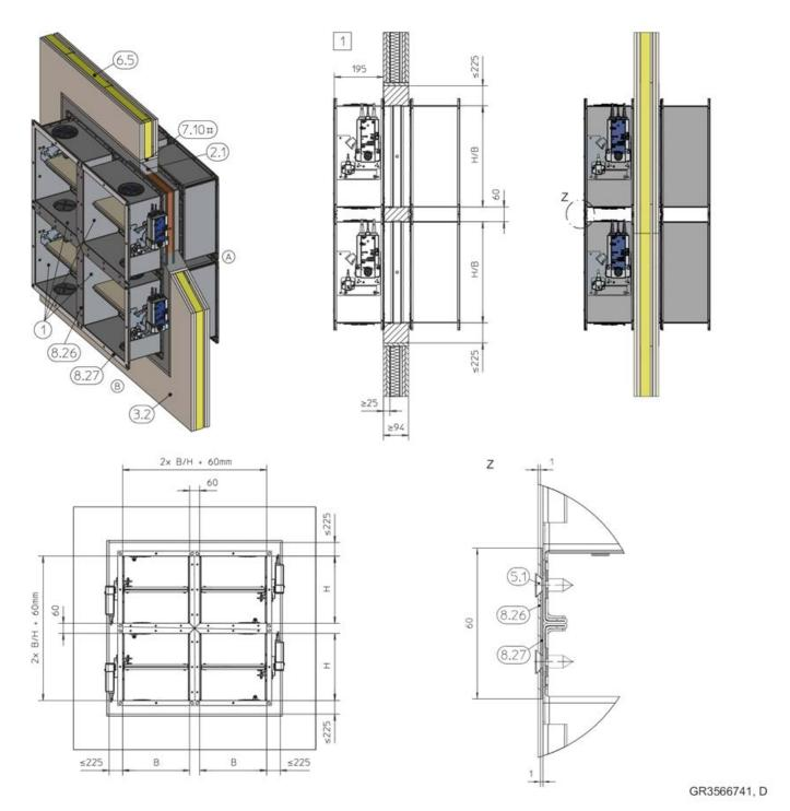
Fig. 78: Mortar-based installation – 4 dampers with a common duct
