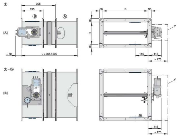
Fig. 6: FKA2-EU with Siemens spring return actuator
