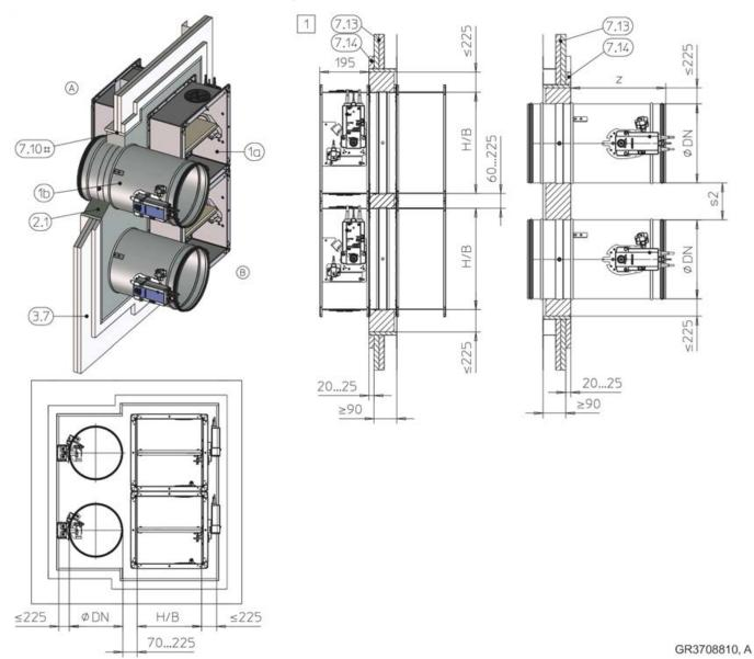
Fig. 125: Mortar-based installation into a shaft wall, FKA2-EU and FKR-EU combined
