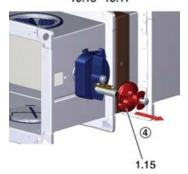
Fig. 179: Removing the fusible link holder
