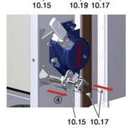
Fig. 182: Removing the fusible link holder
