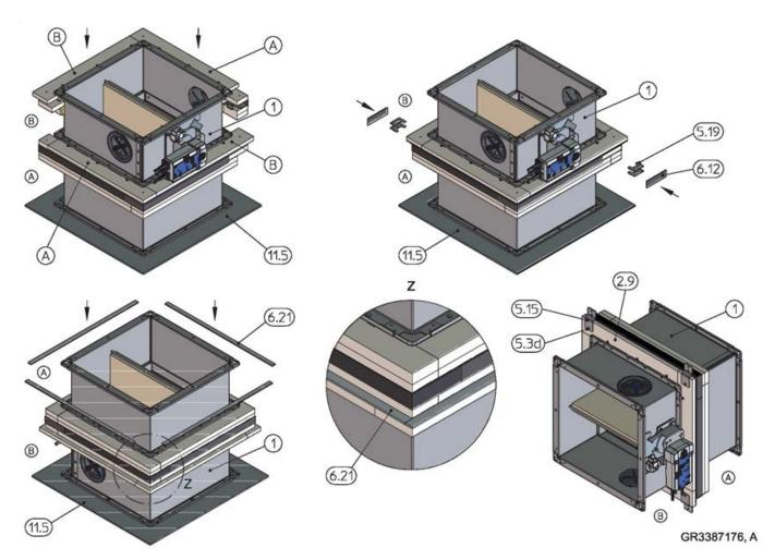
Fig. 33: Installation kit ES for dry mortarless installation - assembly
