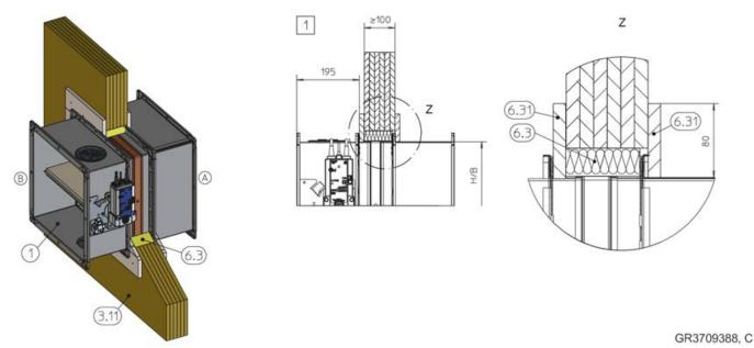
Fig. 118: Dry mortarless installation into a solid wood or CLT cwall, with mineral wool
