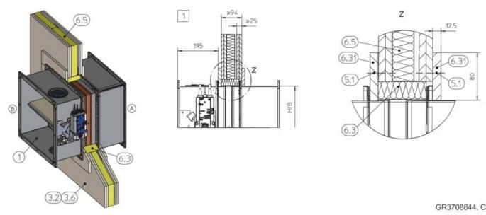
Fig. 82: Dry mortarless installation into a lightweight partition wall, with mineral wool
