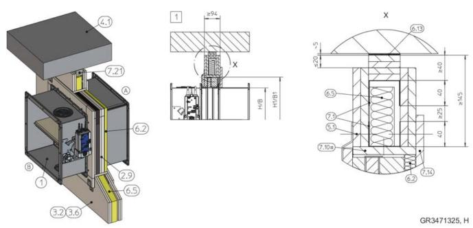
Fig. 81: Dry mortarless installation into a lightweight partition wall, below a flexible ceiling joint
