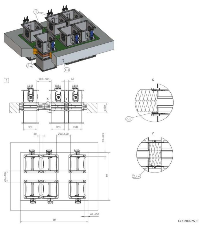
Fig. 150: Dry mortarless installation with fire batt into a solid ceiling slab, multiple installation, flange to flange, illustration shows upright installation (applies also to suspended installation)
