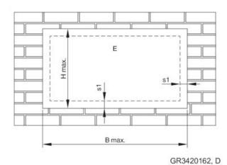
Fig. 29: Fire batt – installation in solid walls and ceiling slabs, lightweight partition, timber stud wall, half-timbered construction and solid wood walls
