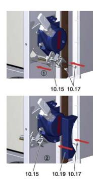
Fig. 184: Install the fusible link holder
