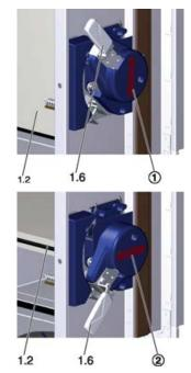
Fig. 171: damper blade position indicator
