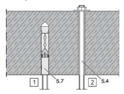
Fig. 157: Fixing to the ceiling slab
