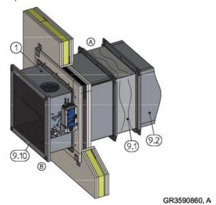
Fig. 164: Fire damper with cover grille
