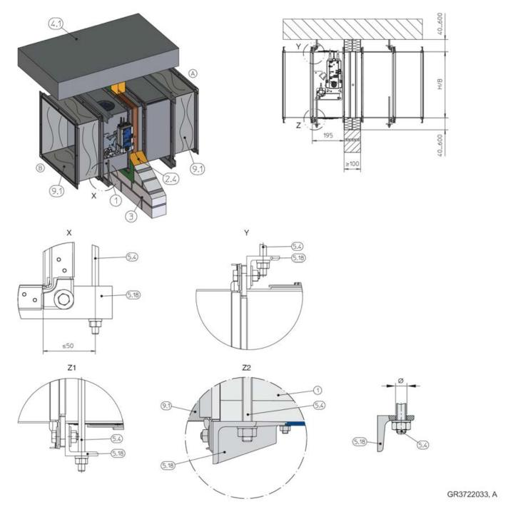
Fig. 159: Fixing of FKA2-EU, wall installation with a fire batt
