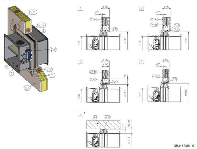
Fig. 105: Dry mortarless installation into a lightweight partition wall with timber support structure, with installation kit ES
