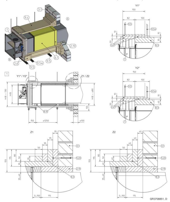
Fig. 57: Dry mortarless installation remote from solid walls with installation kit WE (wall attachment)
