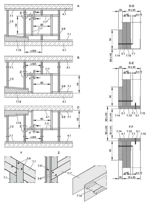
Fig. 121: Shaft wall with metal support structure and cladding on one side (detailed views shown with W = 90 mm)
