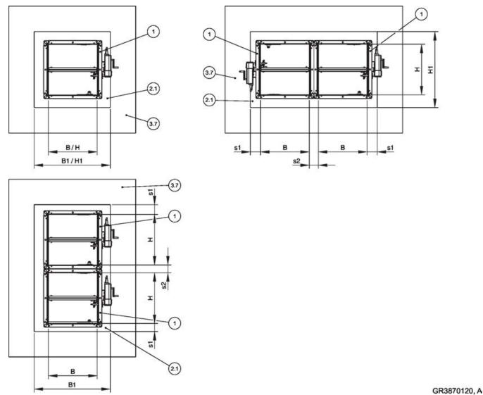
Fig. 120: Lightweight partition walls with metal support structure – arrangement/distances
