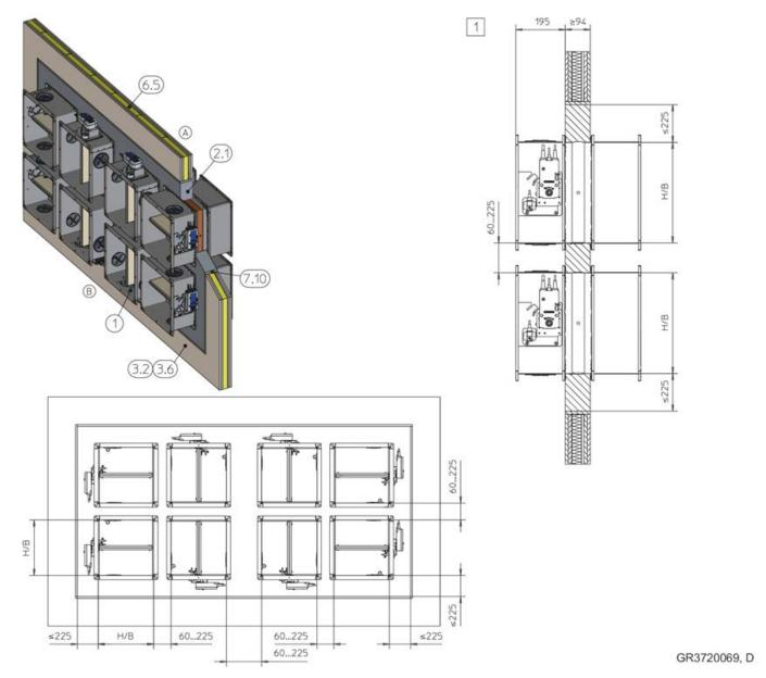
Fig. 76: Mortar-based installation - multiple installation into one installation opening
