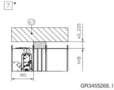
Fig. 122: Mortar-based installation into shaft wall with metal support structure
