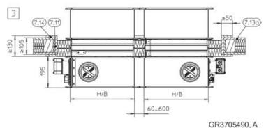
Fig. 110: Dry mortarless installation into a lightweight partition wall with timber support structure, with a fire batt, flange to flange, illustration shows side by side installation (applies also to installation of dampers on top of each other)
