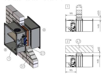
Fig. 44: Mortar-based installation into a solid wall
