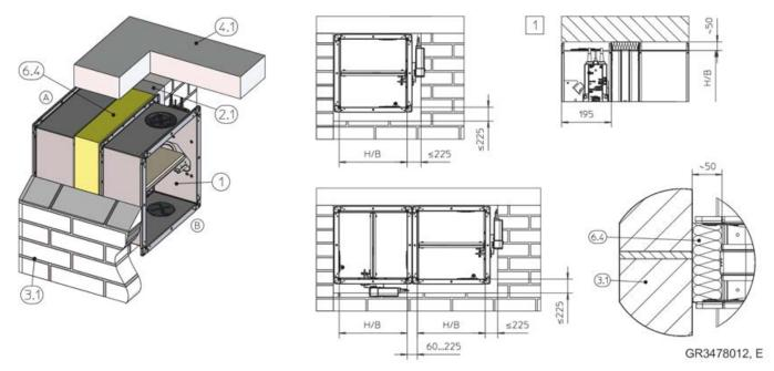
Fig. 54: Mortar-based installation into a solid wall, with partial mortaring
