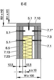
Fig. 66: Compartment wall with metal support structure and cladding on both sides
