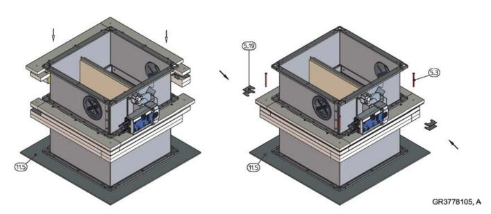
Fig. 36: Installation kit WA for dry mortarless installation – assembly
