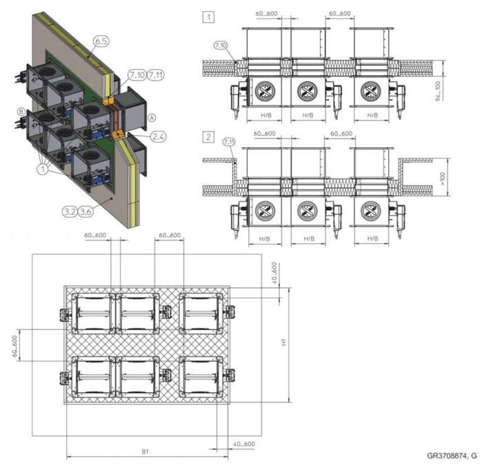
Fig. 88: Dry mortarless installation into a lightweight partition wall, with a fire batt, multiple installation, flange to flange, illustration shows side by side installation (applies also to installation of dampers on top of each other)
