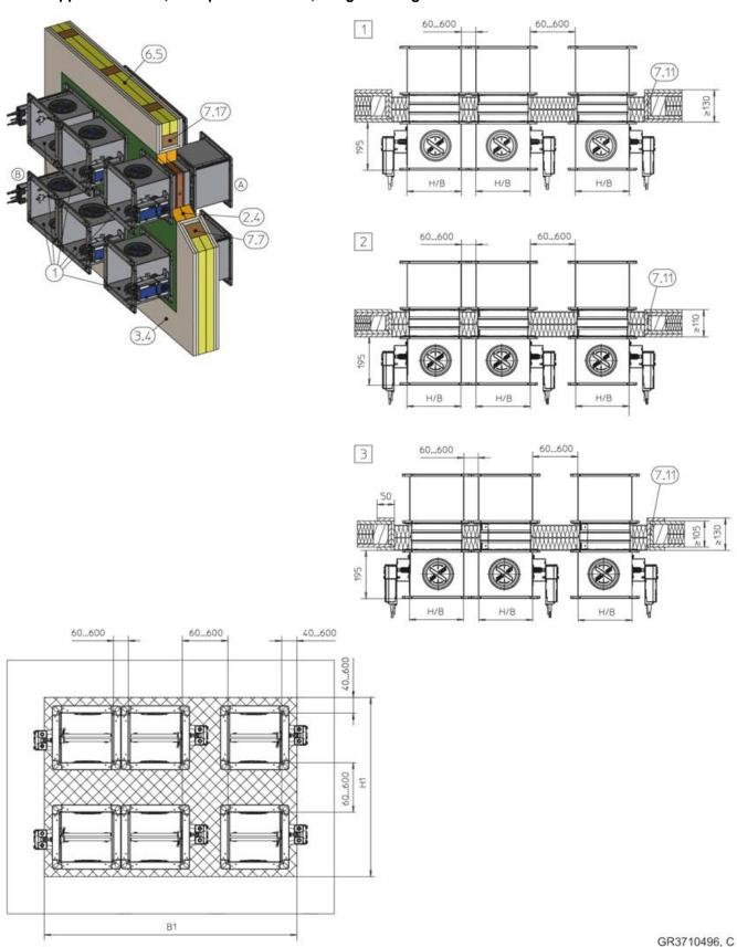
Fig. 113: Dry mortarless installation into a lightweight partition wall with timber support structure, with a fire batt, multiple installation, flange to flange, illustration shows side by side installation (applies also to installation of dampers on top of each other)
