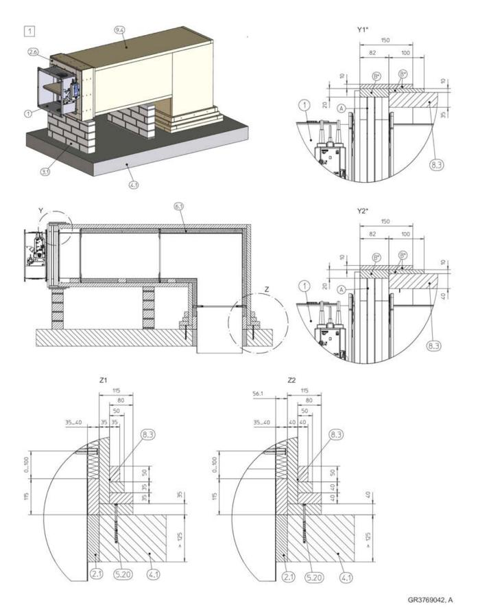
Fig. 147: Dry mortarless installation remote from solid ceiling slabs, with installation kit WE
