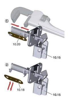
Fig. 183: Replacing the fusible link
