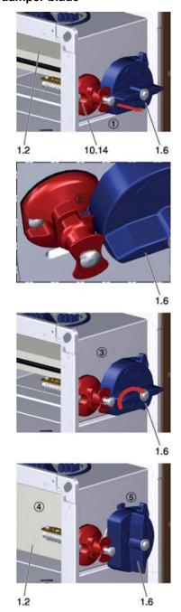
Fig. 169: Close the damper blade
