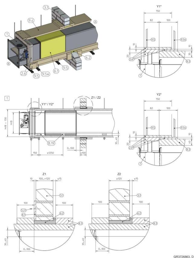
Fig. 59: Dry mortarless installation remote from solid walls with installation kit WE (wall penetration)
