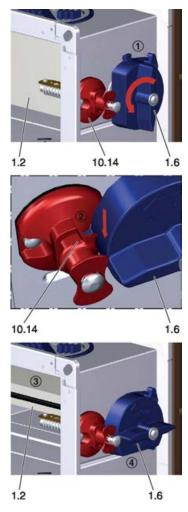
Fig. 170: Opening the damper blade
