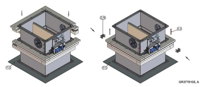
Fig. 40: Installation kit WE for dry mortarless installation – assembly
