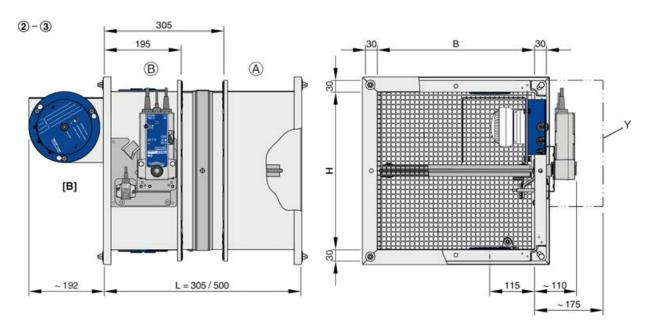
Fig. 10: FKA2-EU with spring return actuator and duct smoke detector as air transfer damper – variant with bracket on the drive side, top right (shown for sizes 2 and 3)
