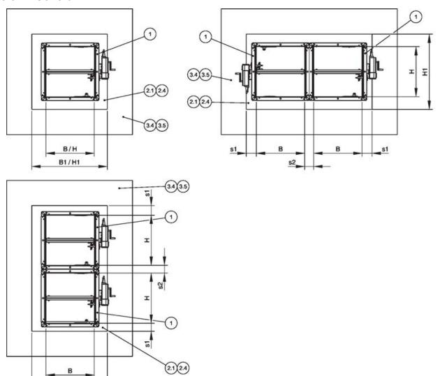
Fig. 89: Solid walls - arrangement / distances
