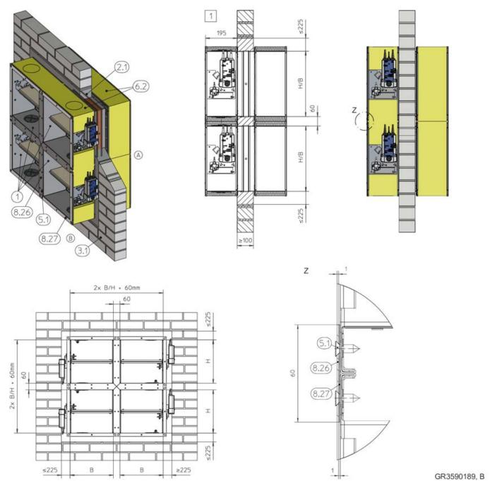
Fig. 52: Mortar-based installation – 4 dampers with a common duct
