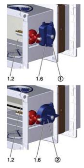
Fig. 168: damper blade position indicator
