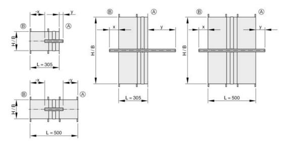
Fig. 161: Open blade protrusion
