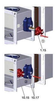
Fig. 181: Install the fusible link holder
