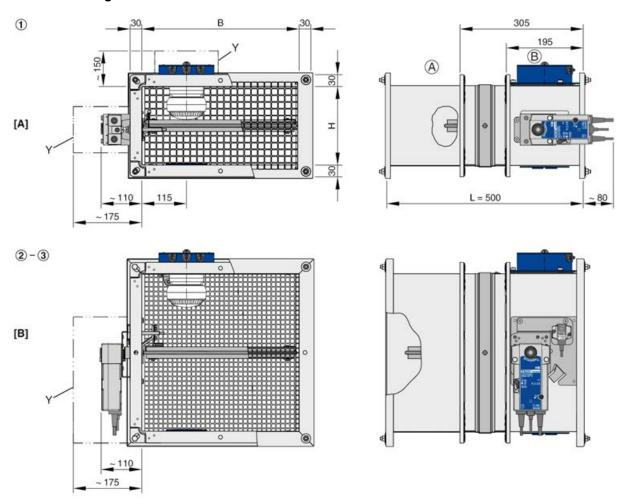
Fig. 9: FKA2-EU with spring return actuator and duct smoke detector as air transfer damper
